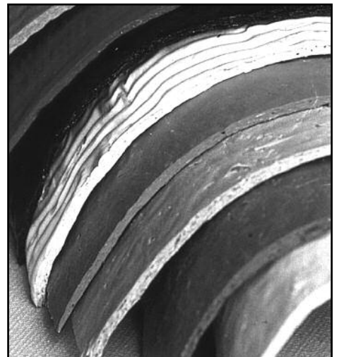
Figure 3. IDI SMC can be formulated with 10 – 60% glass content depending on the physical requirements of the application
